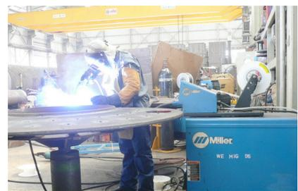
Welding with MIG flux core/CO2 the best method for quality welding.
